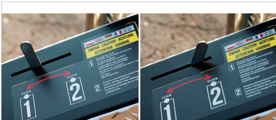
Gear: POSITION 1 - driving/lowering, POSITION 2 - raising
