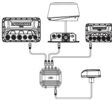
If the number of ethernet devices exceeds the number of available ports on the NEP-2, it is possible to link two or more NEP-2 modules together to provide the required ports. The NEP-2 modules are fitted with 5 ethernet ports. See page 31 for cable options.
