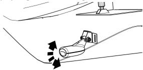
→ Note: A transducer that is tilted too far in either direction will not perform well, missing targets, and/or losing the bottom at speed.
