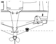
→ Note: Ensure the entire bottom surface of the transducer hangs at least couple of millimetres (1/16ths of an inch) lower than the bottom of the hull.
