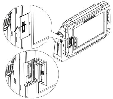
The card reader door should always be shut immediately after inserting or removing a card, in order to prevent possible water ingress.
