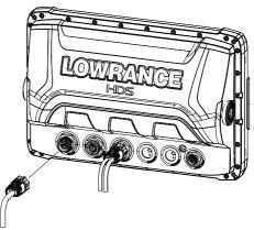
Connector attached to cable is keyed and can only be inserted in one orientation. Once inserted, turn locking collar to secure.
